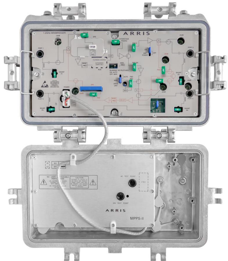
MB120 with 27 dB Return Gain Shown
