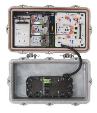
The DT4250 and DT4600 digital return path transceivers support multiple user-selectable modes of operation: a single return ("1-fer") or dual independent returns ("2-fer"). The DT4250 supports bandsplits of 5–42 MHz, 5–65 MHz, and 5–85 MHz. The DT4600 supports bandsplits of 5–85 MHz and is required for 5–204 MHz return.
